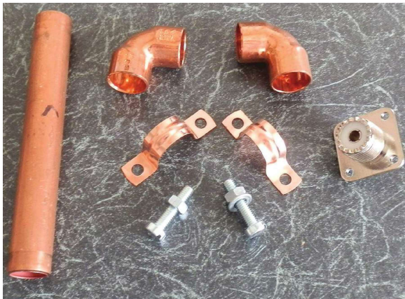
PHOTO 2: Main parts used to make the J-Pole antenna. You will, of course, need rather more copper tube than is shown here.
